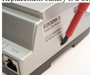
Press the clips on each sides of the box with a little screwdriver to open the top of the box.
