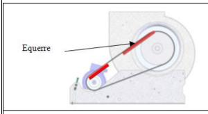
At commissioning, check pulleys' alignment (both motor and impeller pulleys !) along with belt tension.
