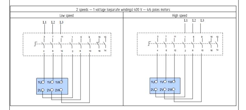
Once wiring is done, check if the impeller is turning in the right direction. If not, reverse two phases and check again.
