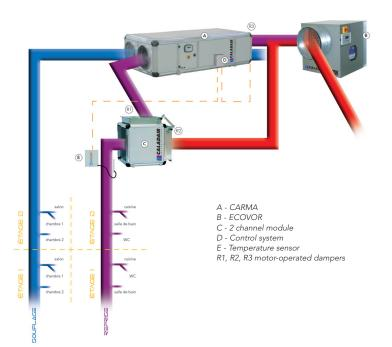
stale air or smoke extraction 1 duct temperature sensor to be positioned in the top of each riser. (option) 1 module 2 motoroperated valves 1 control system (Hardwiring mounted on the station)
