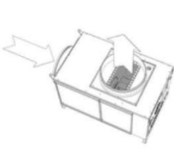
On line intake and vertical exhaust.
