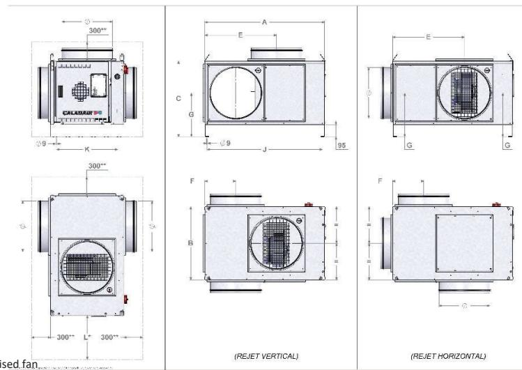
\*Minimum space required to remove the motorised fan.
